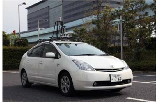
Fig. 1. Vehicle with LIDAR on roof
